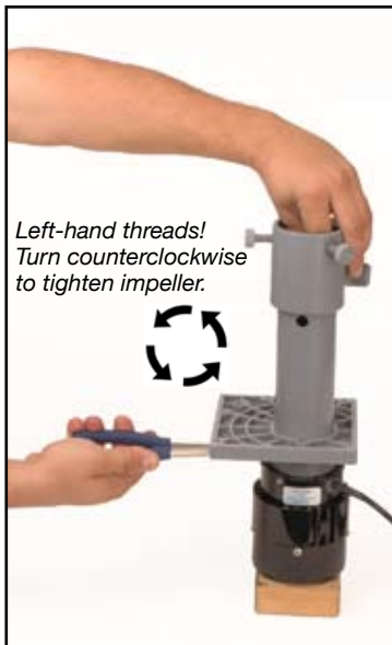
Fig. 13 —Use needle-nose pliers to hold Shaft. Turn Impeller counterclockwise to tighten.
