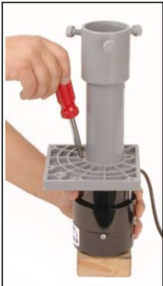
Fig. 12 —Re-install screws through Pump/Motor Base and Spacers.
