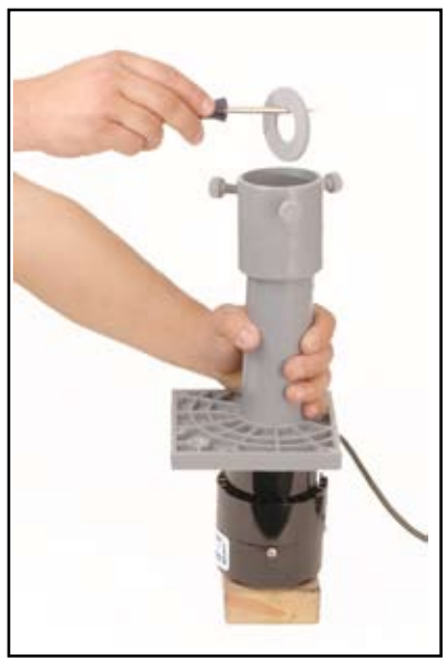
Fig. 4 – Remove Flow Plate and put aside for reassembly later.
