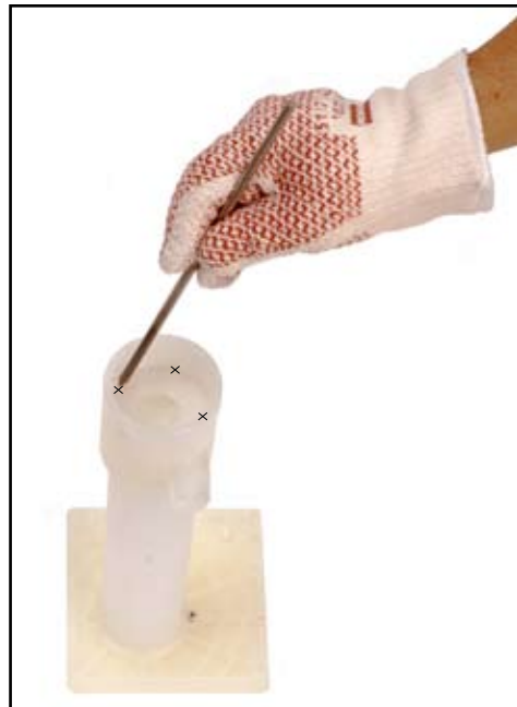
Fig. 17—Touch hot end of object to three locations shown above. This will "weld" Flow Plate onto pump body.
