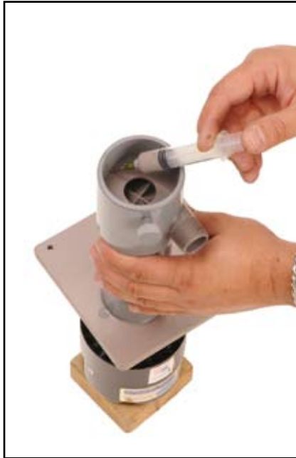
Fig. 15—If pump runs smoothly, reinstall Flow Plate. If you have a CPVC pump (gray in color), use syringe to apply a few drops of CPVC cement around top of Flow Plate. Allow to dry overnight before using pump.
