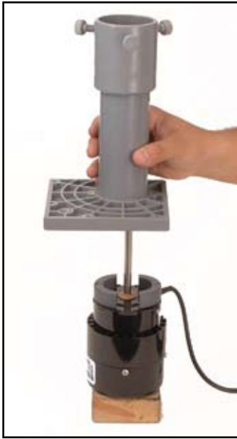
Fig. 10 —Place Base/Body/Housing Assembly over Shaft.
