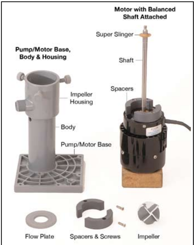
Fig. 2 – Parts identification.
