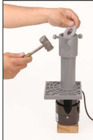
Fig. 14 —Reinstall Flow Plate by lightly tapping with hammer. Then test pump.
