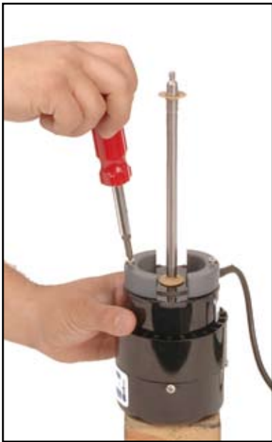
Fig. 9 —Use Phillips-head screwdriver to remove two screws from Spacers.
