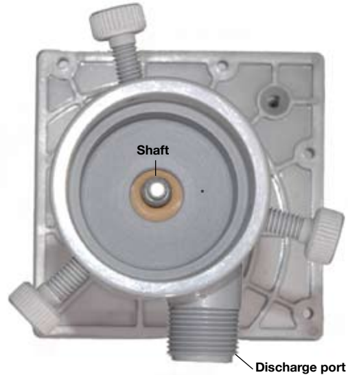
Fig. 11 —Looking down into Impeller Housing, make sure Shaft is approximately centered in hole, as shown.
