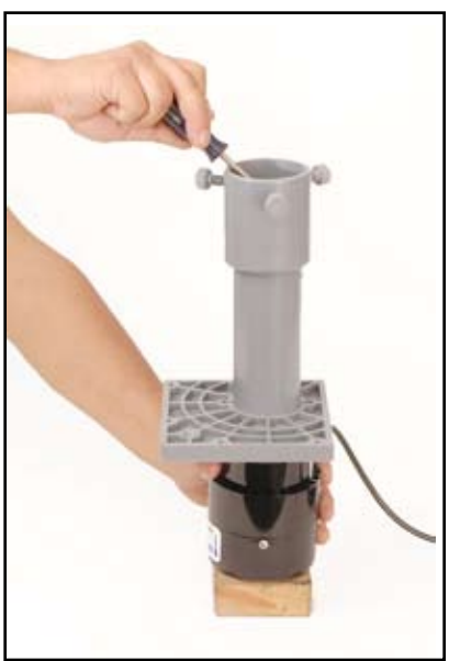
Fig. 3 – Pry out Flow Plate. Be careful not to break!
