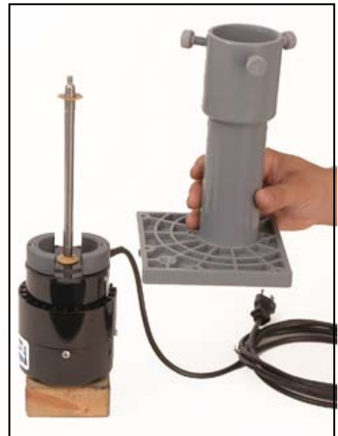
Fig. 8—Remove Base/Body/Housing Assembly.
