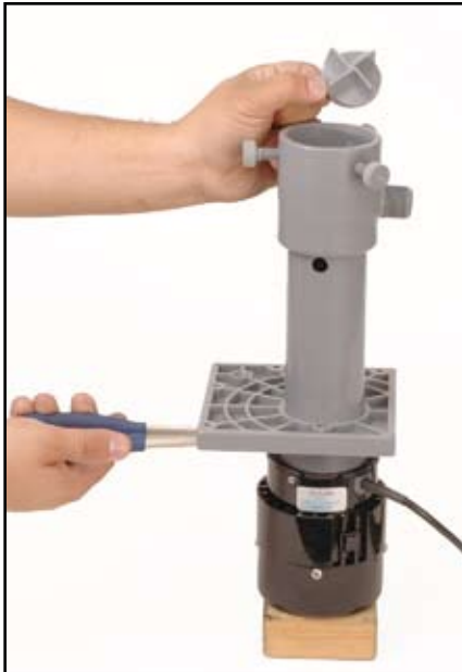
Fig. 6—Remove Impeller from Shaft and put aside for reassembly later.
