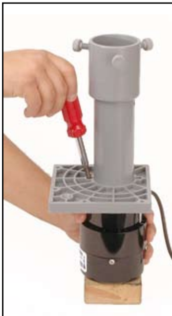
Fig. 7—Remove screws from Pump/Motor Base.
